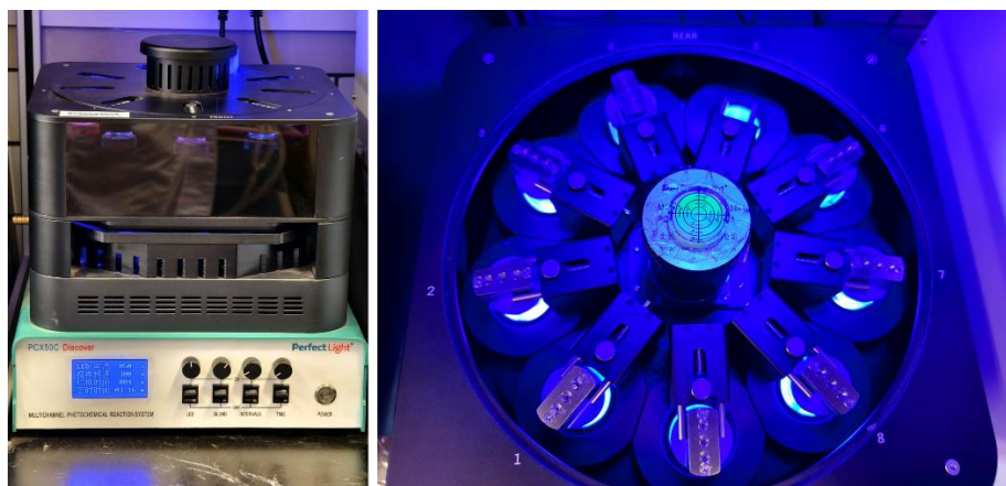
Figure S10. Photocatalytic equipment used for photocatalytic carbon dioxide reduction.
