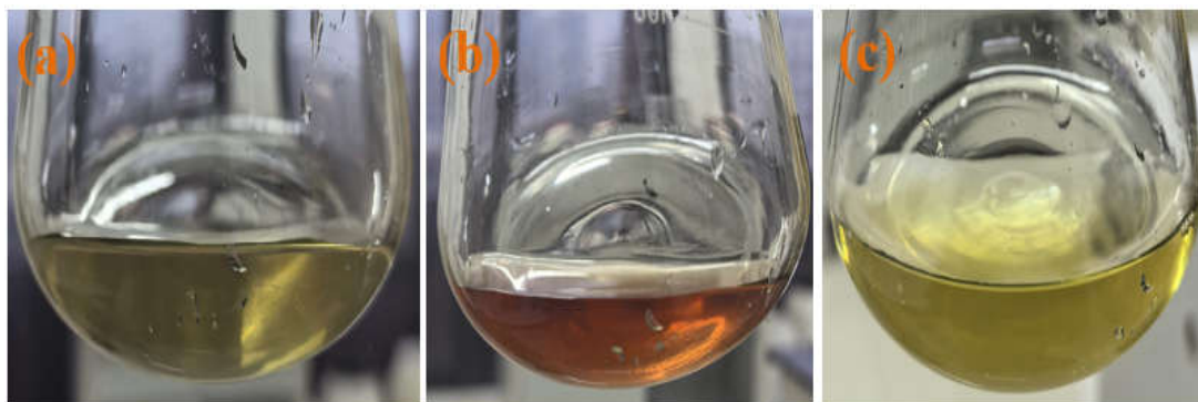
Figure S32. Titration experiments: (a) the color of the catalyst in hydrochloric acid solution, (b) color after addition of xylenol orange, (c) color of the solution at the titration endpoint.
